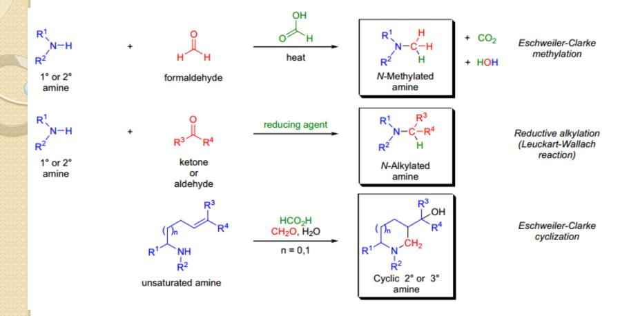
Hydride donor: Formic acid Sodium borohydride, sodium cyanoborohydride, NaBH<sub>3</sub>CN-Ti(Oi-Pr)<sub>4</sub>, NaBH(OAc)<sub>3</sub>, borohydride exchange resin (BER)
